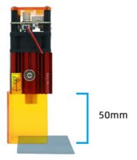
Slide up and down to adjust the focus, find the position of the smallest light spot, the light spot appears as shown in the figure. (Because less power, is more difficult to observe, requires patience adjustment)
