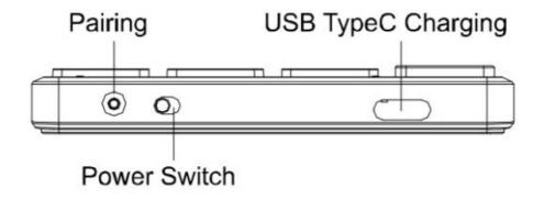
PS: 1. Paring will stop when not paired, if needed, press the Pairing key for pairing again. 2. Power Switch: turn on shows green.
