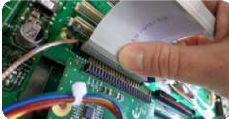
Figure 7: Ribbon cable installation
