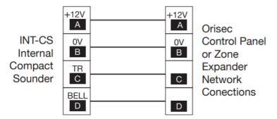
For full functionality connect the INT-CS to the Network Connections on an Orisec alarm system.
