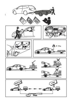
Always refer to the instructions of the vehicle manufacturer, such as the vehicle manual and WVTA, relating to the maximum Permissible towing weight and the maximum vertical ball loading when using the towbar. Ask your vehicle manufacturer / local dealer about maximum towing weights that apply to your vehicle. You must not exceed the relevant specifications.
