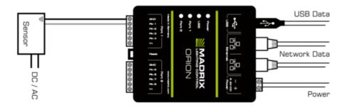
**Description:** Power is supplied to ORION and supplied separately to the input equipment. The sensor is connected to Port 1 via GROUND and DATA at Pin 1, but <u>not</u> V+!
