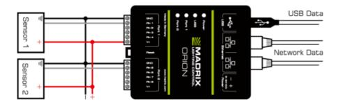
**Description:** 5 V - 24 V power is supplied externally and to all input equipment. For example, a sensor is connected to Port 1 via GROUND, DATA at Pin1, and V+ to supply power to ORION once, while a second sensor is connected to Port 2 via GROUND and DATA at Pin 5, but <u>not</u> V+!
