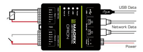
**Description:** Power is supplied only once to ORION and also used for the input equipment. Each Port is protected with 500 mA max. For example, a potentiometer is connected to Port 1 via GROUND, DATA at Pin1, and V+, while a switch is connected to Port 2 via DATA at Pin 5 and V+.
