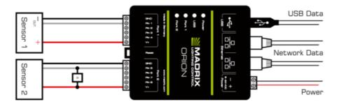
**Description:** Power is supplied only once to ORION and also used for the input equipment. Each Port is protected with 500 mA max. To Port 1, a PNP output sensor is connected over 0 V - 12 V. To Port 2, an NPN
