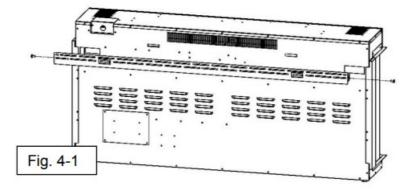
• After you have selected a suitable location for wall mounting, locate the studs on the wall. You must be able to secure to a minimum of 2 studs for proper installation of the bracket.
