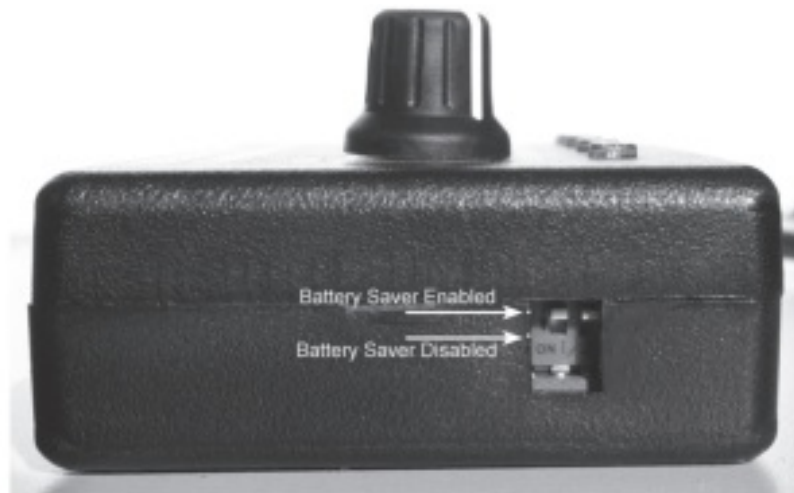
Figure 4. Move Switch 1 to the down position to disable the battery saver. Switch 2 is not used.
