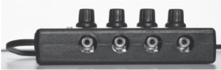
Figure 3. Each of the four the control knobs controls the jack aligned with it.
