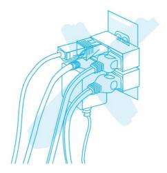
• Do not pull the power cord to disconnect from power source. Always grasp the plug to pull out.
