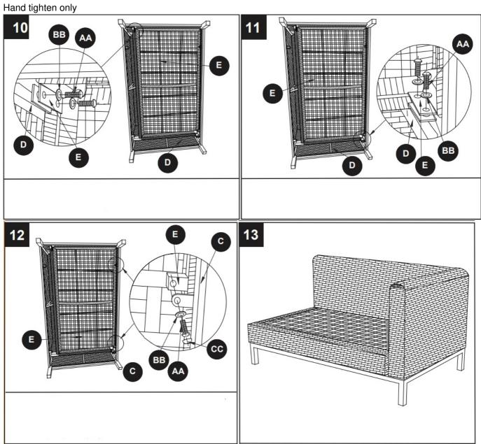
Once assembled, securely tighten all bolts with ratchet wrench (DD), then cover all bolts with bolt covers (CC).
