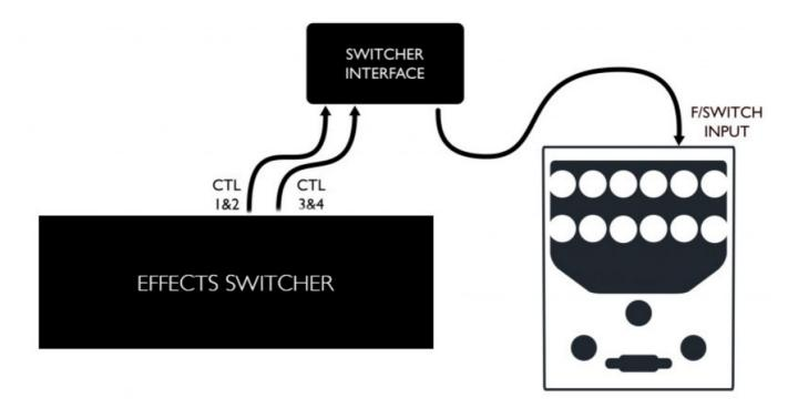
**NOTE:** Remote switching of the bypass state and active channel can only be achieved with the Switcher Interface. The interface converts latching control formats to a short momentary pulse. In the unlikely event of power loss, the user may find that switcher-to-pedal synchronization is lost. To re-sync the setup the user should toggle the affected function directly on the pedal, by pressing the appropriate footswitch.
