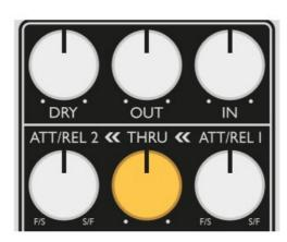
**IN:** This control sets the level into the first compression stage. Higher settings result in more compression, as more signal is pushed over the fixed threshold. The LED on the right will indicate when the first stage is compressing. Increasing the IN control will also make the signal louder, so this should be balanced with the THRU and OUT controls.
