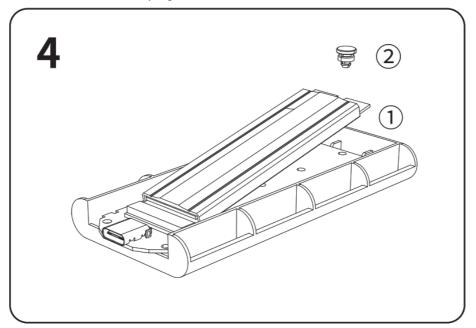
Put the SSD tray in and the top cover back and tighten the screw.
