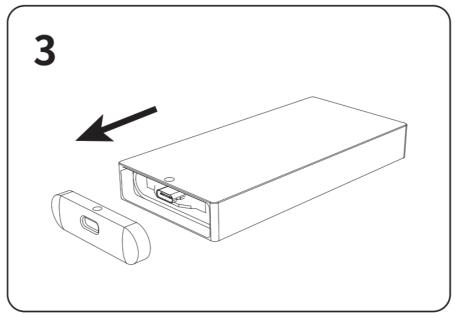
Insert SSD in and fixed SSD with silicone plugs.
