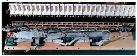
Now solder the switch board wires to the key contacts:
