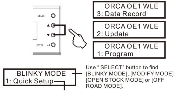
Us ▲e button and " " button to find the right position of the motor link.
