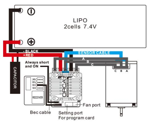
Position the ESC where it is protected in the event of a crash. Use the supplied double sided tape to secure the ESC to the chassis.
