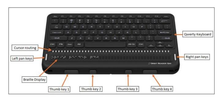
The normal operating orientation of the device is with the four Thumb keys closest to you. Above the Thumb keys is the line of braille cells. On the left and right side of the braille line are two buttons. These buttons are used to skip to the next or previous line of braille and are known as the pan keys.
