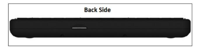
. At the bottom of the device, is the switch to Power cut-off of the device.
