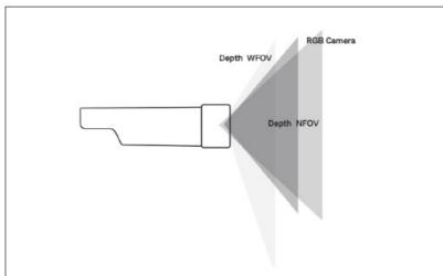
This image demonstrates the camera's field-of-view as seen from the front at a distance of 2000 mm. When depth is in NFOV mode, the RGB camera has better pixel overlap in 4:3 than 16:9 resolutions.
