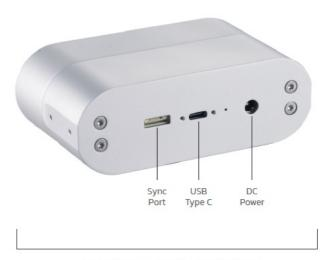
Femto Bolt rear-view showing interfaces
