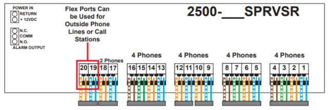
For 28-36 zone systems, two Supervisor Boards are included. Wire as shown below
