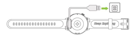
Connect the charging cradle to a power supply, the device's screen will light up and display the battery level.
