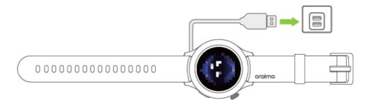
Wipe the metal contacts, and the device dry before charging.
