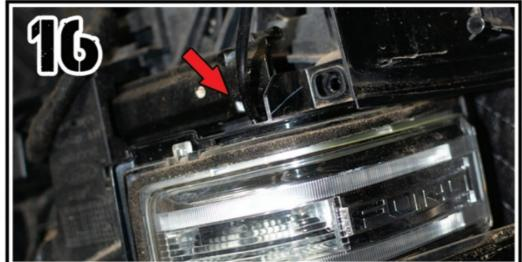
THE CABLE FOR THE MIRROR CAPS WILL RUN BEHIND THE TURN SIGNAL HOUSING. NOW REASSEMBLE MIRROR IN REVERSE ORDER.
