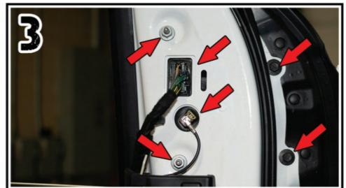
NEXT, DISCONNECT THESE TWD PLUGS AND LOOSEN THE TWO 10MM NUTS AND 10MM BOLTS.
