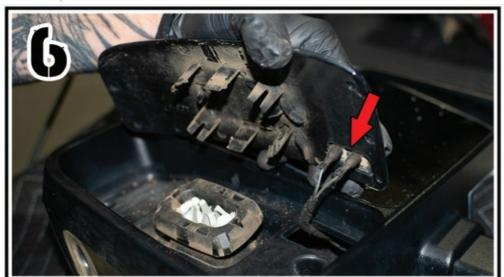
DISCONNECT THESE TWO MIRROR HEATER PLUGS FROM THE MIRROR GLASS
