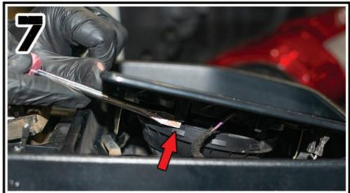
USING A FLAT HEAD SCREWDRIVER, DEPRESS THESE CLIPS TO DISCONNECT THE UPPER MIRROR GLASS.
