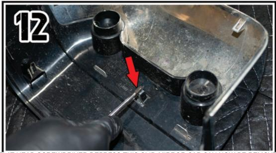
USING A FLAT HEAD SCREWDRIVER.DEPRESS THIS CLIP. MIRROR CAP CAN NOW BE REMOVED.
