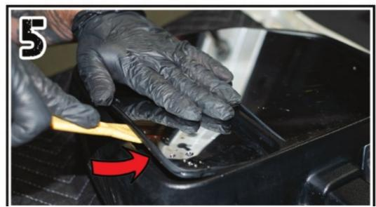
USING A PANEL TOOL, REMOVE THE LOWER MIRROR GLASS BY DEPRESSING THE CLIPS.
