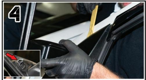
USING A PANEL TOOL, DEPRESS THIS CLIP TO FULLY REMOVE THE MIRROR.
