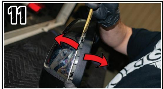
USING A PANEL TOOL, PRY THE MIRROR CAP FROM THE MIRROR HOUSING.
