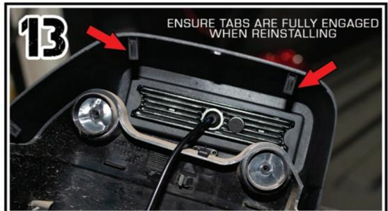
INSTALL THE NEW ORACLE LED MIRROR CAP IN THE PLACE OF OEM MIRROR CAP.
