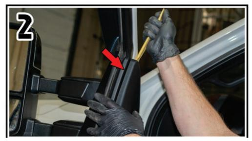
ON THE INSIDE OF THE DOOR, USE A PANEL TOOL TO REMOVE THIS TRIM PIECE.
