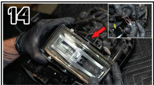
THE POWER PLUG THAT IS CONNECTING TO THIS TURN SIGNAL HOUSING WILL BE USED TO TAP IN OUR WIRES.
