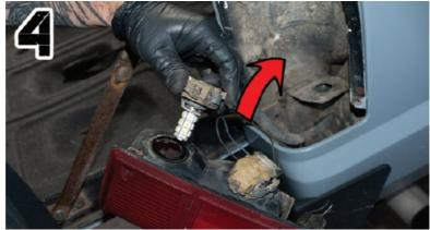
5. START ON THE BOTTOM SOCKET WITH (3) WIRES ONLY. CLIP WIRES FROM SOCKET.
