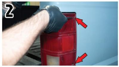
3. NEXT, REMOVE THE (2) PHILLIPS SCREWS ON THE INSIDE OF THE TRUCK BED SIDE.
