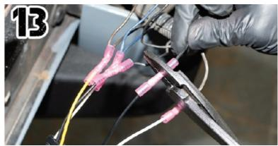
14. HEAT UP THE HEAT SHRINK ON THE END OF THE CONNECTORS. USE A HEAT GUN OR OTHER HEAT SOURCE.
