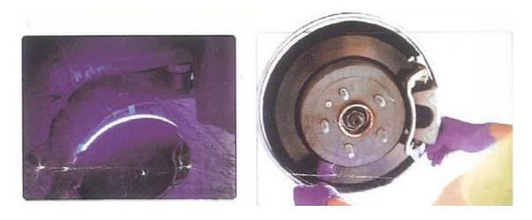
Mock up the light ring in desired location (generally centered around the brake assembly) You snould test your ring before going any further by connecting it a 12 volt battery. While testing check the way the light reflects and mark the ring in the desired location.
