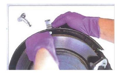
Three mounting brackets will be used for each ring. The pre-drilled hole is where the ring r mounts to the bracket However you will need to drill through the aluminum nng and use the self tapping screws, to drill through the dust shield.
