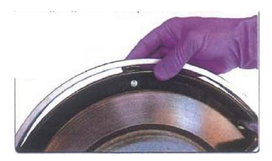
Use the self tapping screws to attach to the dust shield and the bracket at the same lime. This will insure that the bracket is mounted tightly to the Glust shield.
