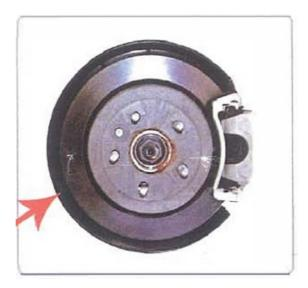
Begin removing the wheel from your vehicle.Behind each brake system is a metal brake dust shield (indicated by the arrow in the oicture.) This is what will be used to mount your LED wheel rings to.
