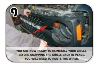
**Step 10** Image: Routing wires under the turn signal.
