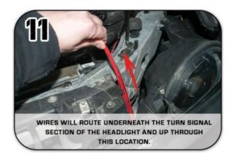
**Step 12**Image: Running wires through the frame.
