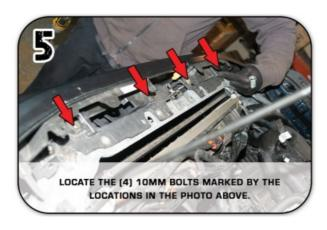
**Step 6**Image: Using a 10mm socket to loosen the bolts. USE A 10MM SOCKET TO LOOSEN THE (4) 10MM BOLTS.
