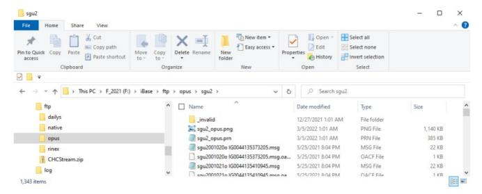
If an OPUS solution is returned that is unreadable, or is superseded by a solution that is newer, better ephemeris then the old solution will be moved to the \_invalid or \_duplicates folder.
