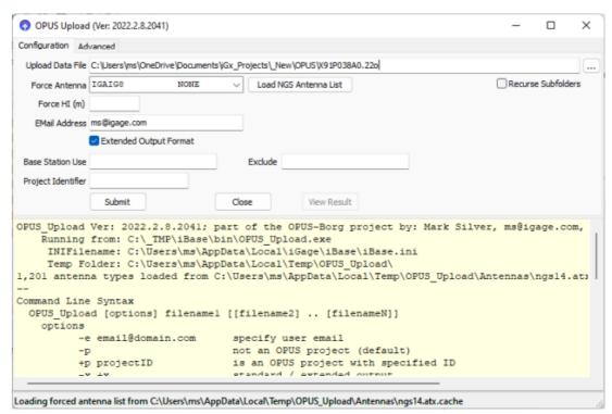
OPUS\_Upload (OU) is a small Win-32 application that automates the submission of GPS observation files to the online NGS processing system. OU navigates the HTTPS NGS website using SSL encryption.
