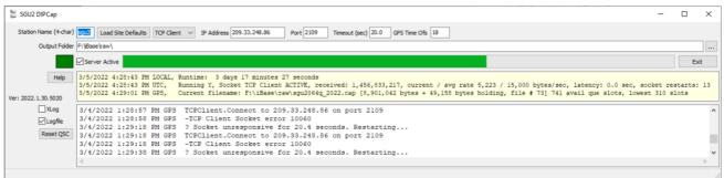
DIPCap is a replacement for RCAPTURE. RCAPTURE fails after a few days or weeks and only supports TCPIP 'Client' connections, DIPCap is very robust and will run forever. It has better logging and also supports TCPIP 'Server' connections.
