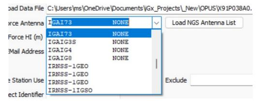
Click on the 'Load NGS Antenna List' button to download the current antenna list file from the NGS server ( <a href="https://geodesy.noaa.gov/ANTCAL/LoadFile?file=ngs14.atx">https://geodesy.noaa.gov/ANTCAL/LoadFile?file=ngs14.atx</a> ). The list is parsed and every antenna, including the satellite definitions, are loaded into the drop-down box in sorted order.
