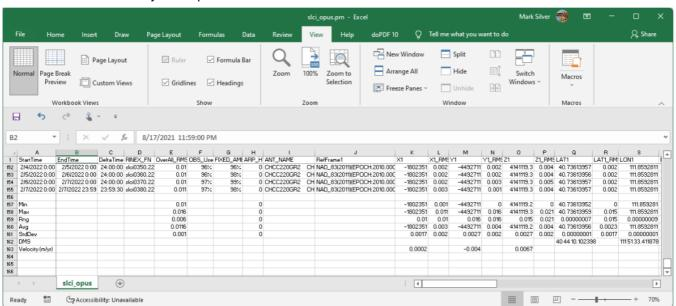
This summary includes an average position for the CORS station along with the Min/Max/Range/StandardDeviation for each of the values found on an NGS OPUS solution.
