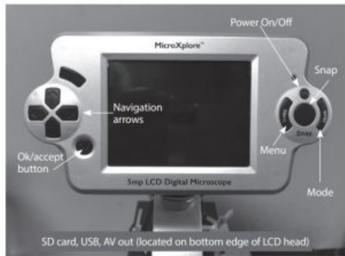
Figure 3. The LCD screen, with power and navigation buttons shown
