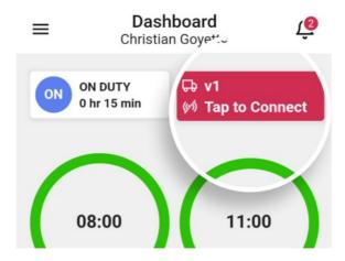
(1) Use **Tap to Connect** bar to connect to your vehicle. The device will attempt to connect to selected vehicle ELD via Bluetooth. ELD bar will change from red to orange: **Pairing**
