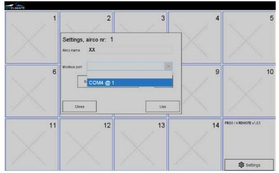
• At this dialog you can selection the modbus-port and set the airco name. Use the 'help' button to show the possible dip-switch setting of the airco. You can set the modbus-port-address with the dipswitch of the airco.
