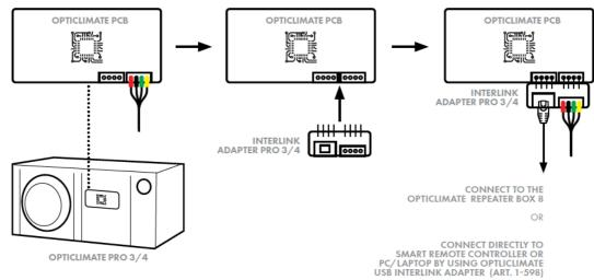
Control 1 Opticlimate remotely: Connect the USB Interlink Adapter to the USB-port at the Smart Remote Controller (or Computer). Use a Black Interlink Cable and install an Interlink Adapter PRO3/4 in your Opticlimate to connect the USB Interlink Adapter with your Opticlimate PRO3 or PRO4.
