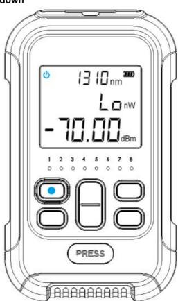
After pressing briefly , the meter will turn on and start the automatic shutdown function. The default automatic shutdown time is 10 minutes. If you want to cancel the function, press and hold the power key for two seconds,
