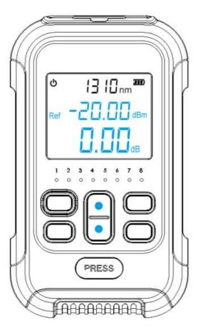
After power on, enter the interface of OPM, press REF to set the current power as the reference power, switch the relative optical power test (insertion losstest) and absolute power test. In the relative power test mode, the insertion loss (dB) and the reference value is displayed simultaneously. Short press "dB" to switch linear power and absolute power display. The units of linear power, absolute power and relative power are W, dBm and dB respectively.
