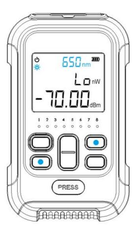
After power on, long press the /VFL key to turn on the VFL, short press to flash and turn off. Press the power button to control the flashlight turn on and off.
