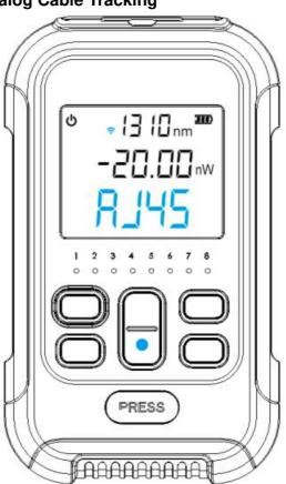
In the test interface of OPM, long press the dB key to display the word "RJ45" on the screen. At this time, enter the RJ45 cable sequence test, connect one end of the network cable to the RJ45 port in the bottom, and connect the other end to the remote tester. Short press the dB key to exit. Long press the dB key again, ""displays on the upper left corner of the screen, enter the cable tracking mode, and short press the dB key to exit.
