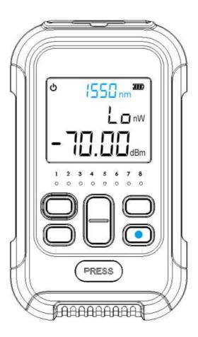
In the interface of OPM, short press the  $\lambda$  key to switch the measurement wavelength. Ten different wavelengths can be selected: 1310nm, 1550nm, 1577nm, 1490nm, 1625nm, 1650nm, 850nm, 1270nm, 1300nm and 980nm. In order to ensure the accuracy of the test, the selected wavelength must be consistent with the measured optical signal.
