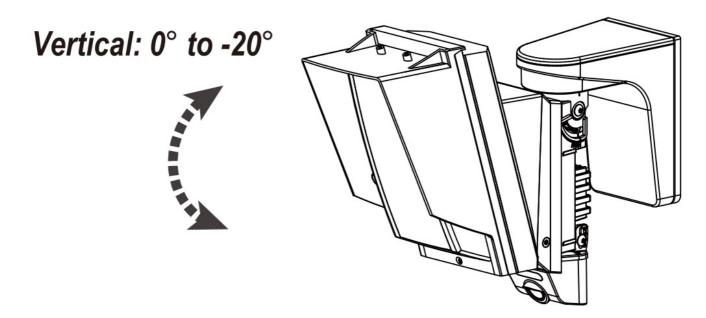
Do not use the vertical angle adjustment of the main unit other than adjusting the detection area surface to be parallel to the ground inclination.
