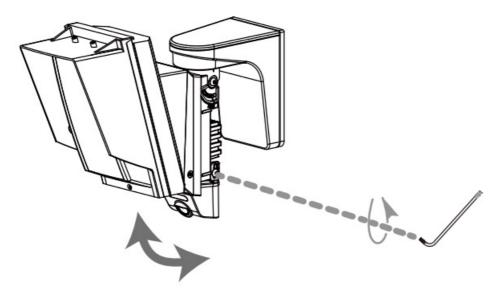
Loosen the screw to adjust camera angle
