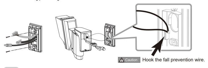
NOTE To pass cables through the wall, drill a 25 mm (1") or larger hole in the wall.
