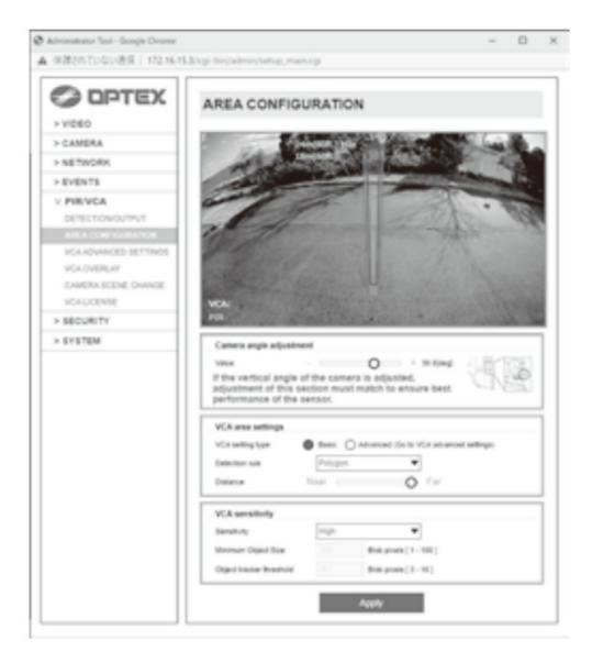
Caution If the vertical angle of the camera is to be adjusted, adjustment of this sections must be matched to ensure the best performance of the sensor.
