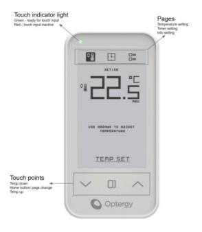
The Wireless thermal stat operates in one of 2 modes: Autonomous and Active.
