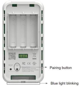
**Step 5:** Press and hold the pairing button on the gateway at the same time as the thermostat, check out for green leds which would mean paired
