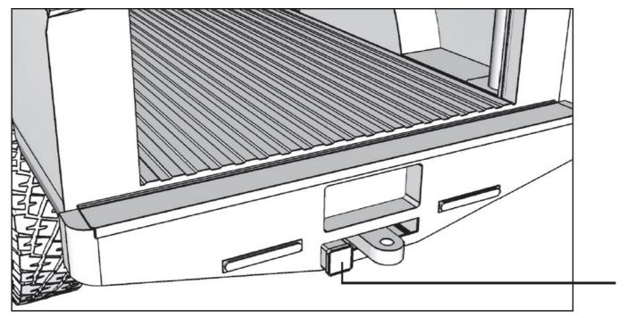
If your vehicle have a 7-way trailer outlet, you can directly connect the "AUX Red Wire" to the "AUX 12V(+)" to power the light bar.
