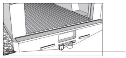
If your vehicle have a 7-way trailer outlet, you can directly connect the "AUX Red Wire" to the "AUX 12V(+)" to power the light bar.
