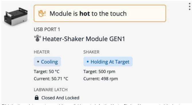
• Click the three-dot menu to reveal the available controls for the Heater-Shaker. You can control the heater, shaker, and labware latch independently. You can also view information about the module, including its serial
