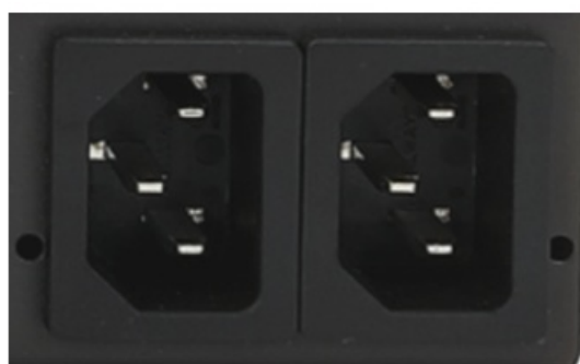
Figure: Dual power supply connectors for CM8100
