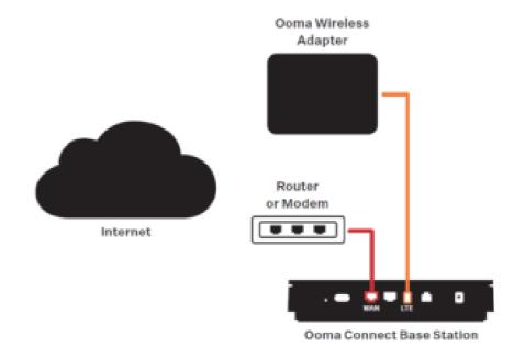
Wireless Adapter can provide either a primary or a backup Internet connection.
