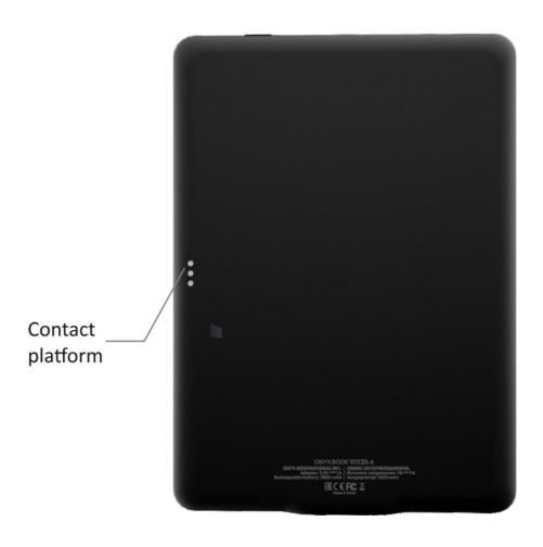
Contact platform Designed to communicate with the buttons of the case
