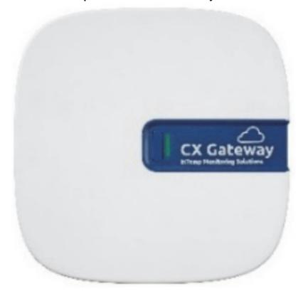
The In Temp CX5000/CX5001 Gateway uses Bluetooth® Low Energy (BLE) to regularly configure and download data from up to 50 CX series loggers and upload the data to the In Temp Connect® website automatically using Ethernet or Wi-Fi. The gateway requires an In Temp Connect website account with gateway privileges and a phone or tablet with the InTemp app installed to set up the gateway.
