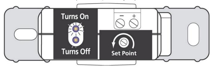
**STEP 1:** Turn the setpoint screw counter-clockwise until the Status Open LED turns off and the Status Closed LED turns on. (Sensor should be in this state right out of the box.)
