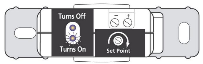
**STEP 2:** Slowly turn the setpoint screw clockwise until the Status Closed LED turns off and the Status Open LED turns on.
