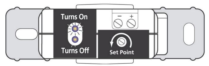
**STEP 2:** Slowly turn the setpoint screw counterclockwise until the Status Closed LED turns on and the Status Open LED turns off.
