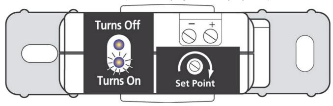
**STEP 1:** Turn the setpoint screw clockwise until the Status Closed LED turns off and the Status Open LED turns on.
