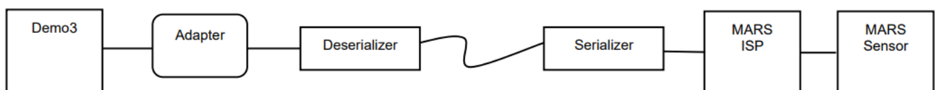
Diagram of MARS ISP and Sensor with SERDES between ISP and Sensor
