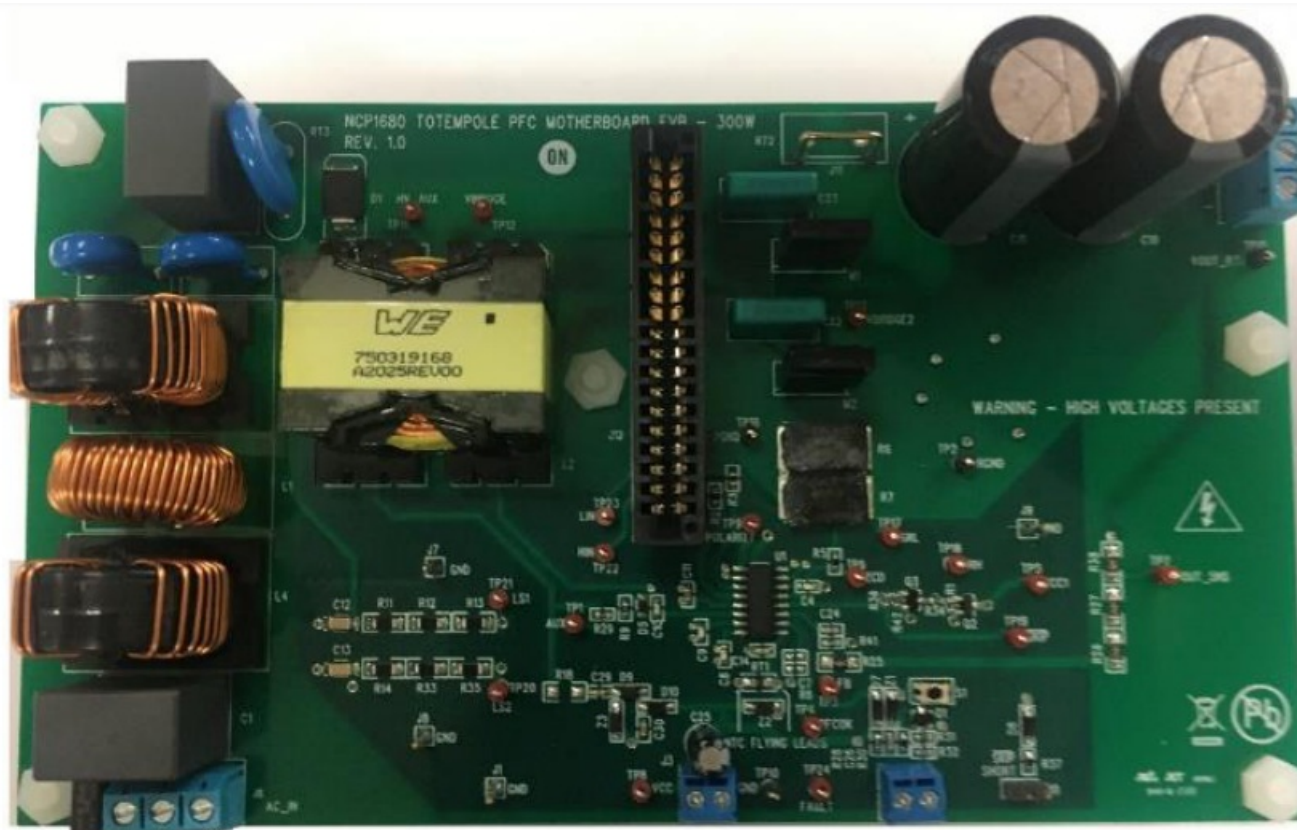
Figure 1. NCP1680 Evaluation Board
