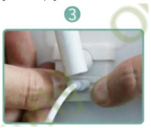
3. Insert the charging cable and firm the rubber stopper.
