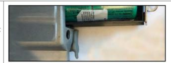
2. Attach the Power Adaptor to the connector plug. As soon as you plug the adaptor into the lock, it will cycle until it is ready to open.
