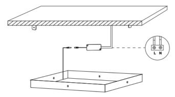
3. Place the frame on bracket and use screws to fix.
