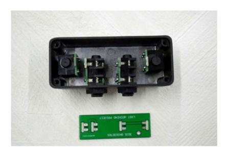
At this time, place the side jack toward you so that the board faces to the left. Align the holes in the main PCB with the protrusions on the four jack boards. Align it so that the side labeled "SOLDERING SIDE" is facing up.
