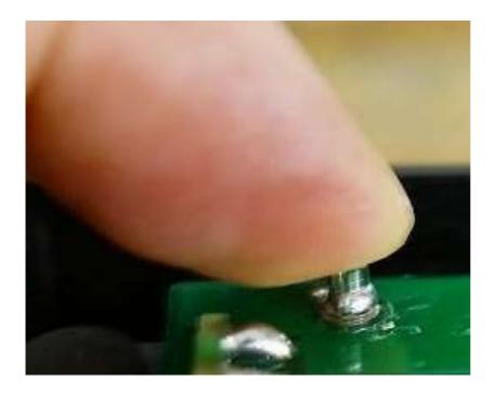
After applying the solder, check that the bar moves. If the bar moves when you press it with your fingers from above, there is no problem.
