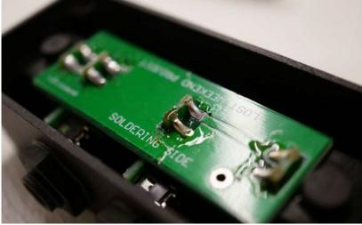
At this point, verify that the top and side terminals each have power. It's a bit noisy as the back is left open and there's no case shielding, but that's fine at this point.
