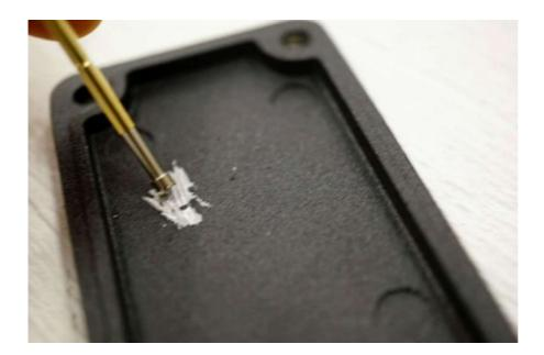
Slightly peel off the paint on the back cover where the ground bar touches.
