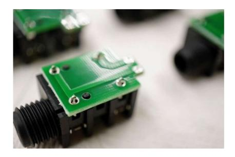
Attach the top jack PCB in the same way, aligning the jack protrusion with the board hole.
