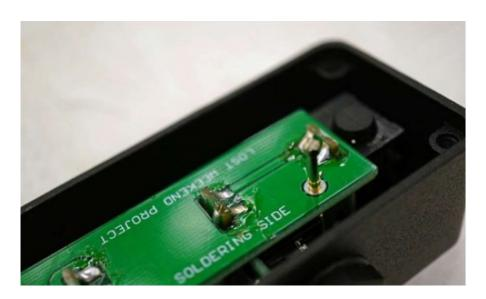
First, thread the ground bar through the hole in the main PCB. Pass the bar until it touches the top of the case, and at that point make sure that the gold part of the bar is sticking out from the PCB.
