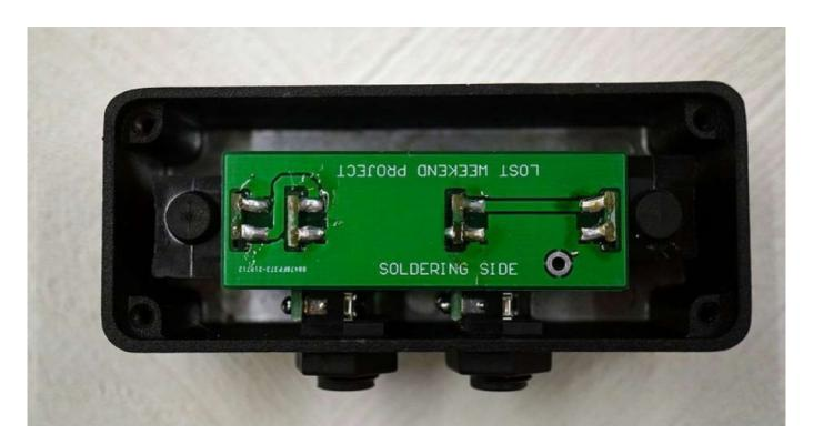
\*If the amount of solder is small, the power may not be applied properly. In particular, apply solder to the extent that the solder penetrates into the eyelet of the jack side board.
