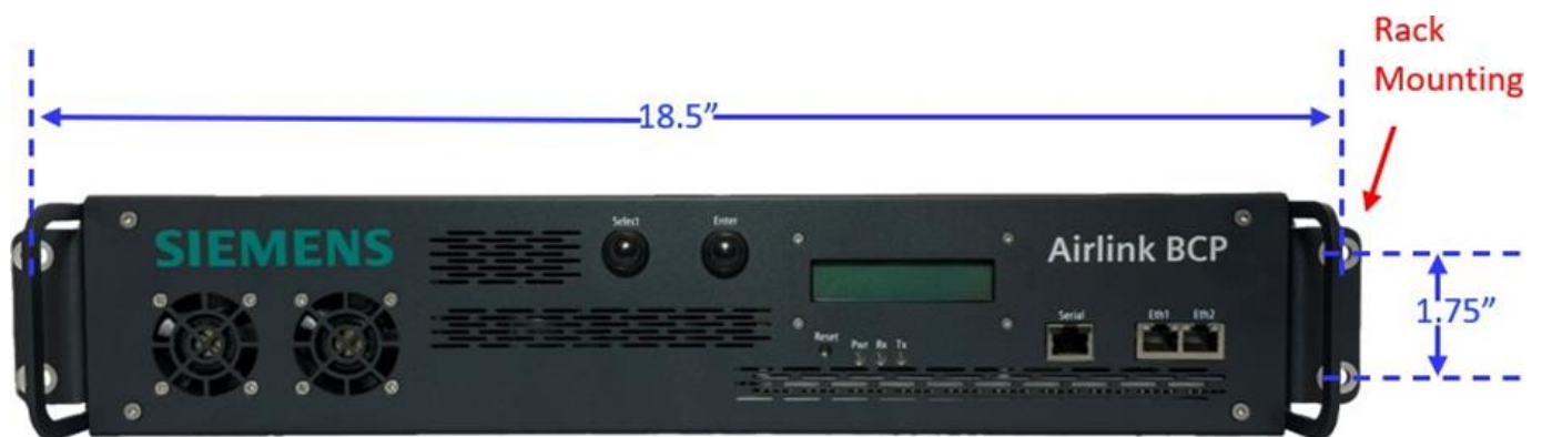
Figure 5 : Airlink BCP Mounting Dimensions
