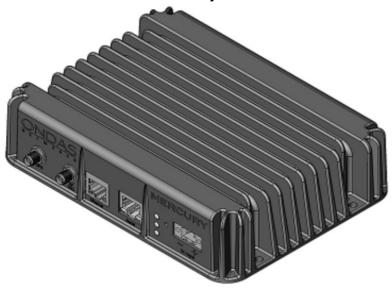
Warning: Never power on a Mercury 450 radio without a load on the RF connector.
