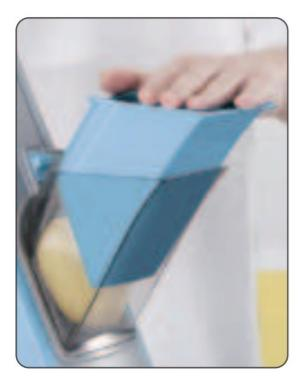
Use the Pusher to guide the ingredient against the Blade.
