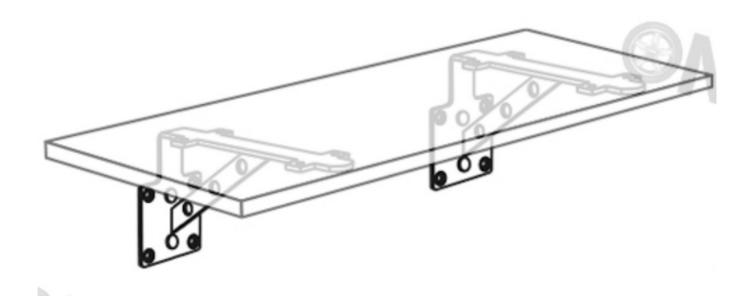
STEP 6: Tighten and secure the board with the short screws
