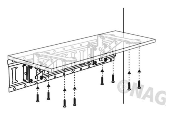
Q: Why do the brackets drop down and are not square to the wall when mated to the E-track?
