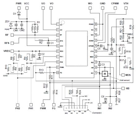
**Notice:** LV 8814J do not include the exposed-PAD The hall sensor is not mounted on the board.
