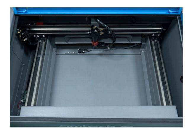
• Step 5. Close the cover. Turn on your control computer, open LaserGRBL or another engraving program, and load your design. You will generally need to click the rotate button shown below, as the engraving forms a mirror image of the displayed design.
