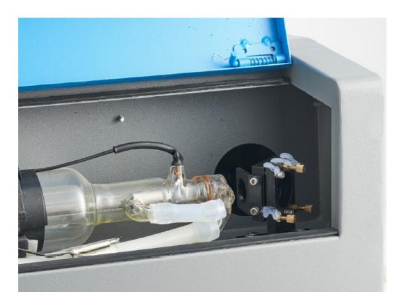
DO NOT place the tape directly onto the mirror. Turn on the machine and set the power level to 11% or lower. Fire the laser. You should be able to see a small mark on the tape. If it is not noticeable, fire the laser again. Always make sure the path is clear between the laser and its target. Never allow foreign objects between the laser and its target. Always close the cover before firing the laser. Do not look directly at the active laser through the cover during this procedure.
