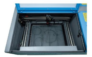
Place a sacrificial base first, preferably a non-reflective steel sheet. Place your laserable material under the laser head and on top of the base, adjusting the base's thickness to make sure the upper surface of the laserable material is at the correct height.
