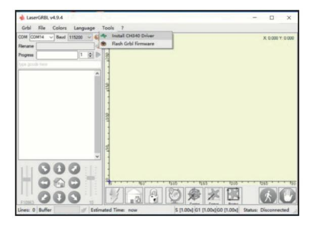
Once the driver is installed, choose the COM port and set the baud rate to 115200. Next, click "Connect".
