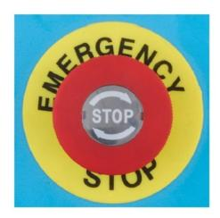
When your engraver arrives, its e-stop should be pressed down and must be released to allow the laser to function. You should test that it works properly before conducting ANY other work with your machine. Start the
