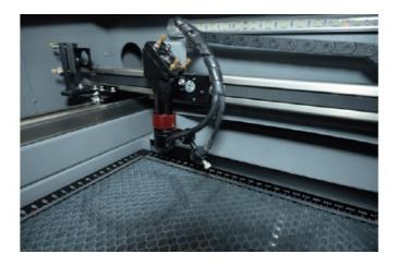
If the distance is too long, you can either move the manual focusing knob down, use a thicker piece of material, or find a safe way to elevate your material to the correct distance. If the distance is too short, move the manual focusing knob up or remove the honeycomb workbed.
