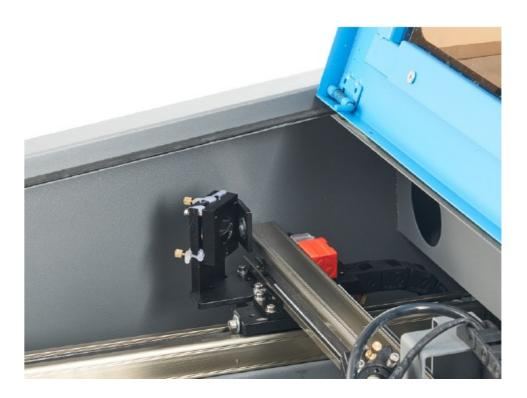
Once set, place a piece of tape on the 2nd mirror's frame. DO NOT place the tape directly onto the mirror. Repeat the steps from §5.3.1. If the laser is not centered on the 2nd mirror, you will need to adjust the 1st mirror's set screws accordingly. For larger adjustments, you may need to loosen the mounting bolts at the mirror's base to slide it into better position before fine tuning with the adjustment screws.
