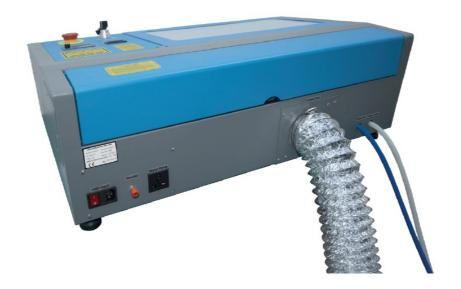
NEVER operate the machine in a closed room and NEVER operate the laser if the vents are not purifying or removing the fumes produced by the target material. Research materials before use and never operate the laser on any (such as PVC, teflon, or other halogen-containing substances) that can produce corrosive, hazardous, or even deadly fumes.
