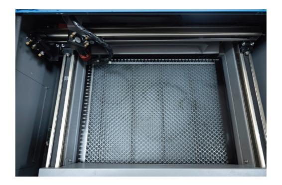
Gently move the laser head along the X axis to the far right. Repeat the steps and adjustments above, again taking care to use the tape on the mirror's frame and not its surface.
